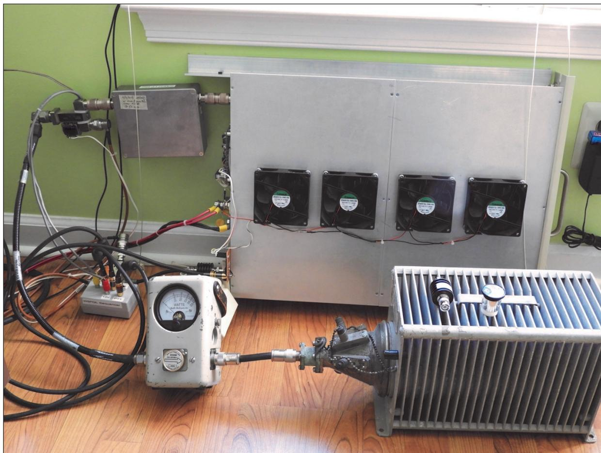
Figure 3. Final Bench Test with amplifier, sequencer, relays, LP filter, dummy load
