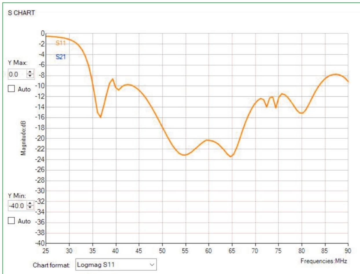
Figure 3. Input into unpowered amplifier modules
